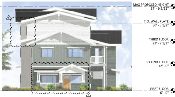
BUILDING B - WEST ELEVATION | 1/8" = 1'-0" | 4
