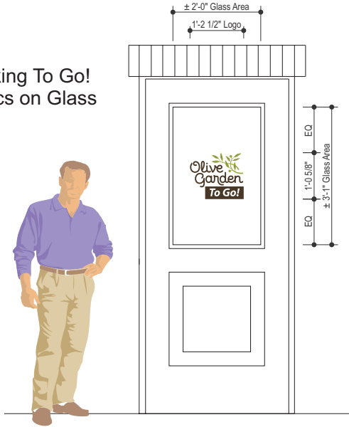
Front View - Carside To Go! Building Entry Door
