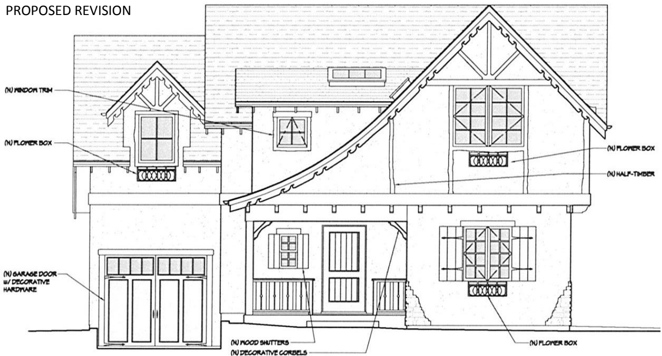
1 WEST ELEVATION SCALE: 1/4" = 1'-0"
